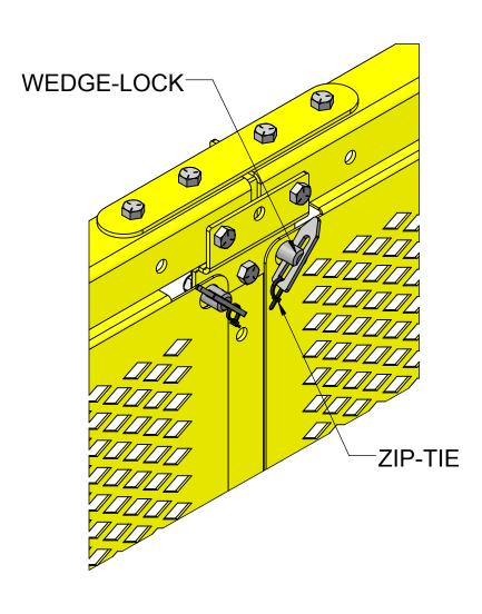
CUT THE TWO (2) ZIP-TIES LOOPED THROUGH THE WEDGE-LOCK ON THE TOP CORNERS OF THE GUARD PANEL YOU WANT TO REMOVE. USE A SIDE-CUTTER OR OTHER APPROPRIATE CUTTING TOOL
