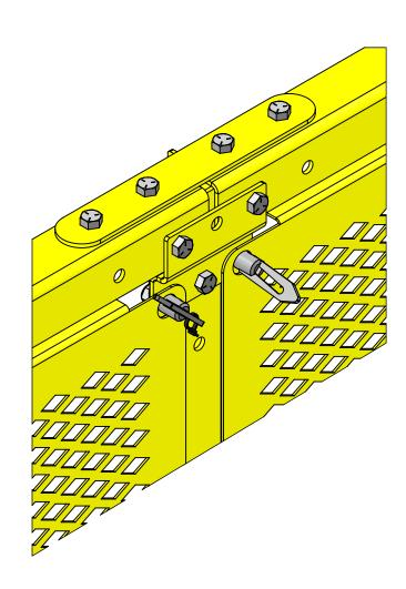
OPEN THE TWO (2) WEDGE-LOCKS YOU JUST REMOVED THE ZIP-TIES FROM. A HAMMER MAY BE REQUIRED TO KNOCK THE WEDGE LOCK LOOSE.
